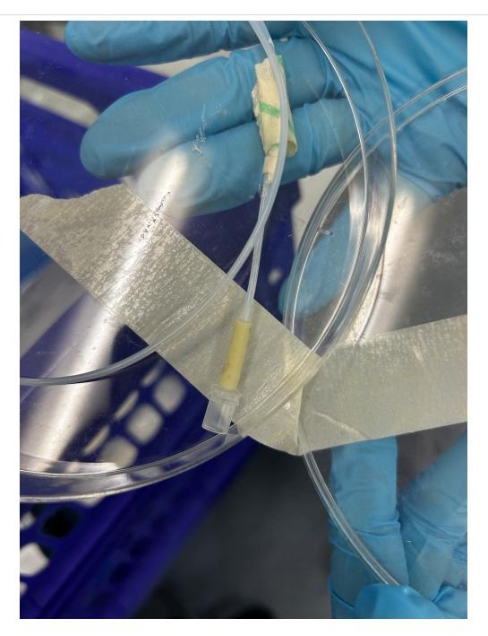
Image of the tubing assembly - this is the end that will connect to the syringe. See Guidelines section for how to prepare the tubings.
