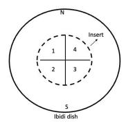
Schematic of Ibidi dish and suggested labelling to ensure correct orientation. N and S must be added both to the lid and the base of the dish in exactly the same positions to ensure correct alignment.
