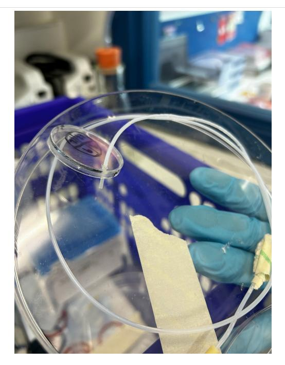
Image of the lid with a hole for the tubing end that will be inserted into the medium with cells. See Guidelines section for how to make the hole in the lid.
