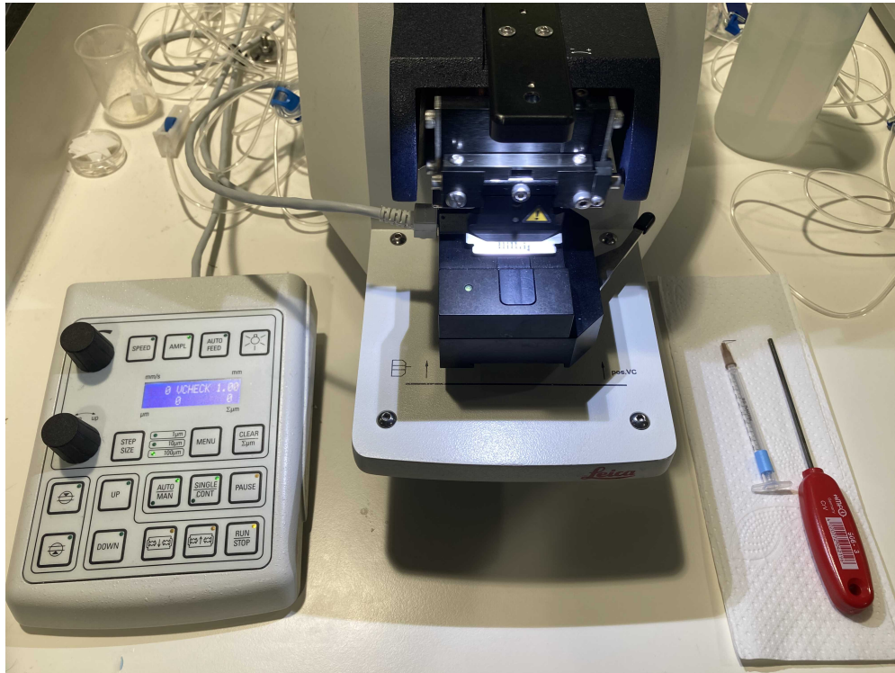
Figure S9. Blade alignment with the Vibrocheck on a Leica VT1200S.
