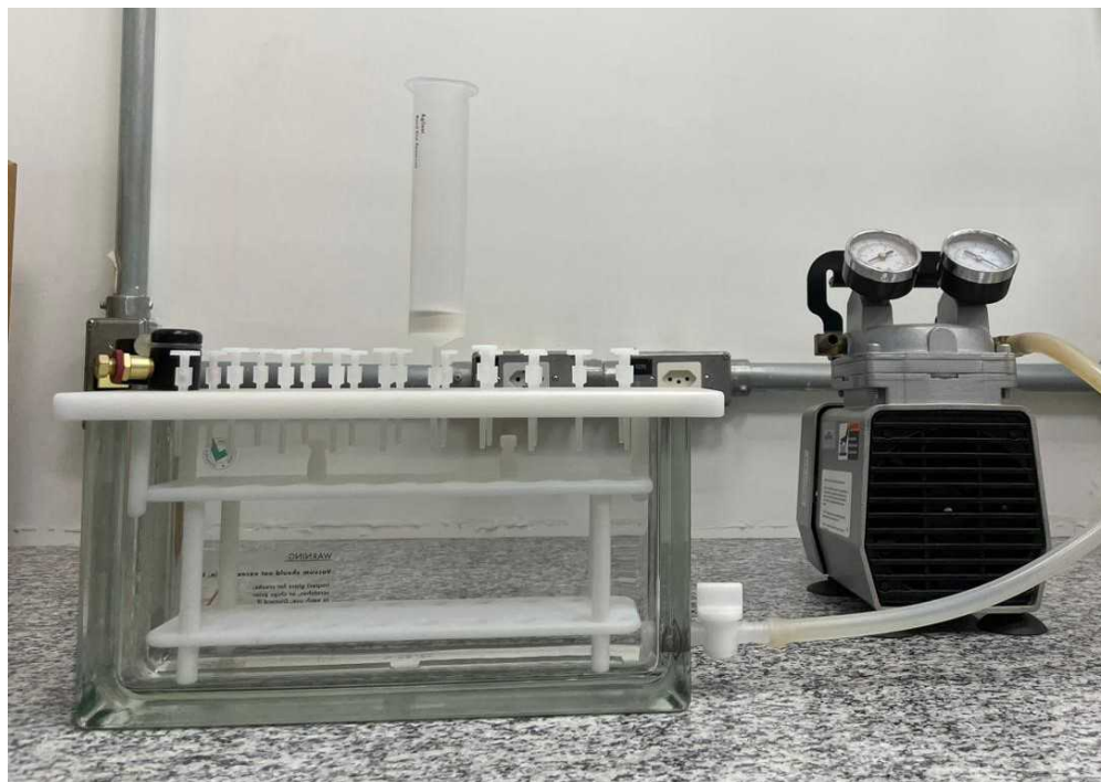
Figure 2: Vacuum manifold with a packed SPE column. Source: Authors (2024).
