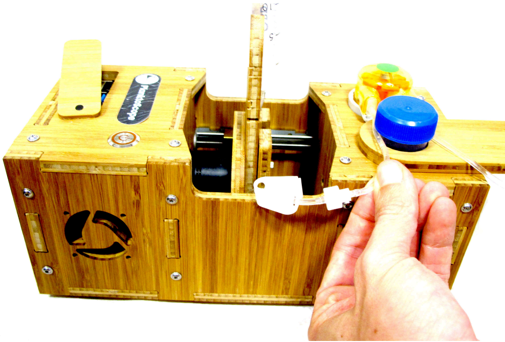
Figure 9: How to unclog the fluidic path. If your fluidic system is not optimized to avoid plankton sedimentation, some plankton could accumulate in the fluidic system. This can be checked by pinching the tube halfway in between the flowcell and the pump during 1-2 seconds (to accumulate suction pressure) and releasing it. If a large quantity of plankton passes suddenly this means that plankton have sedimented between the syringe and the flowcell.
