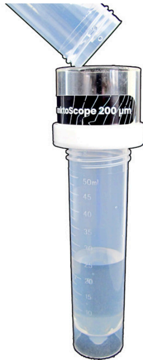
Figure 1: How to filter the sample with the 200 µm sieve.
