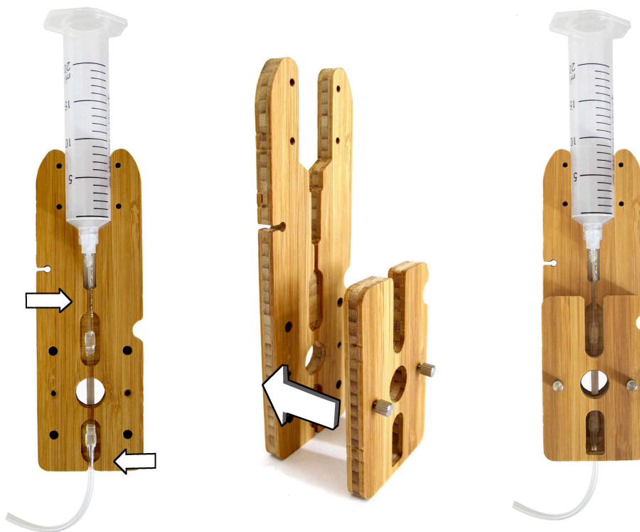
Figure 5 : How to install the flow cell. You will need the syringe (F9), the flowcell receptacle (E) and one flowcell (F7).
