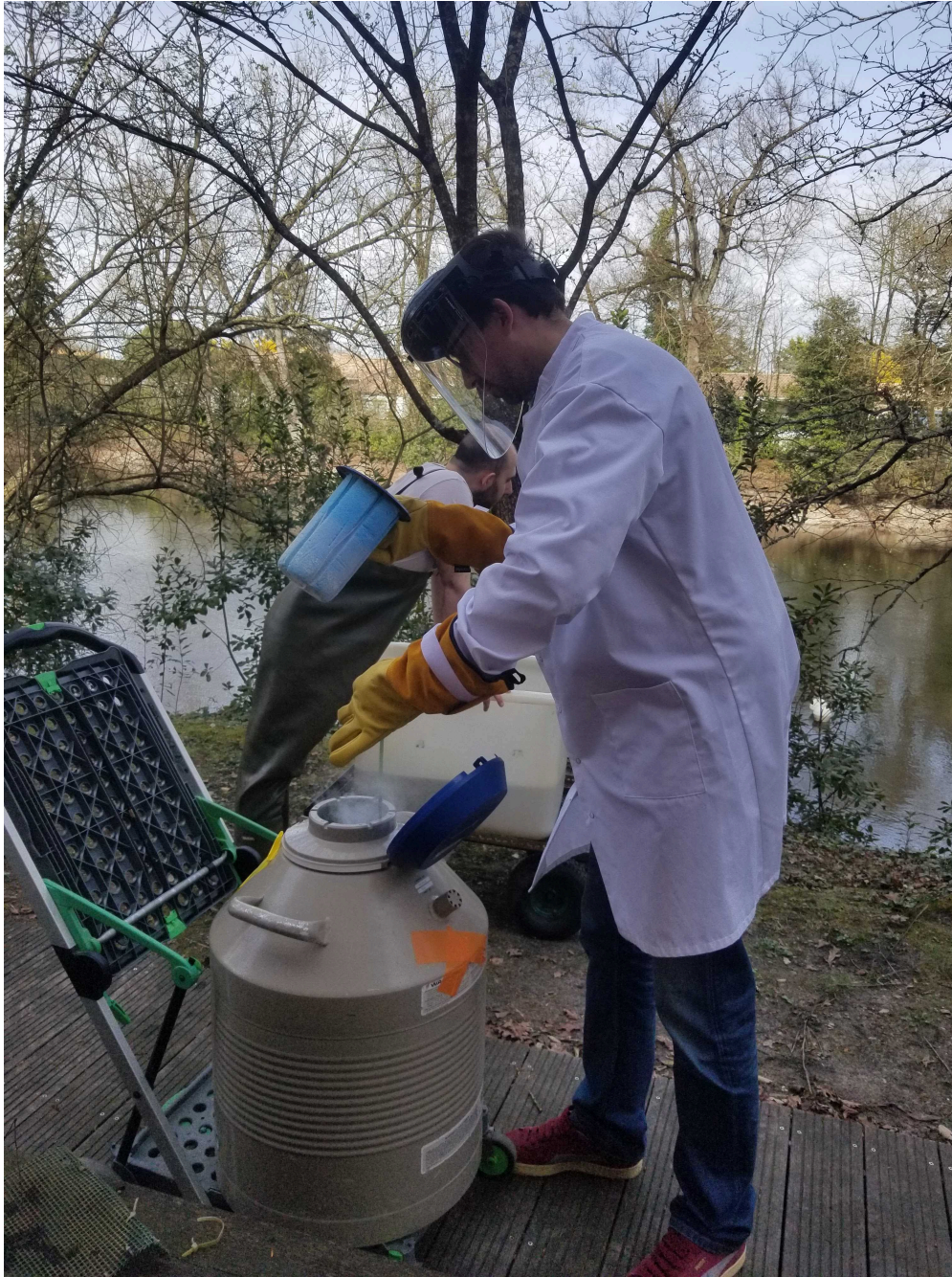
Quenching samples in liquid nitrogen
