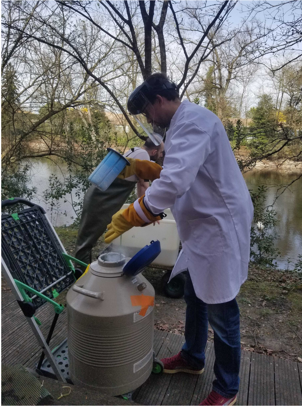
Quenching samples in liquid nitrogen
