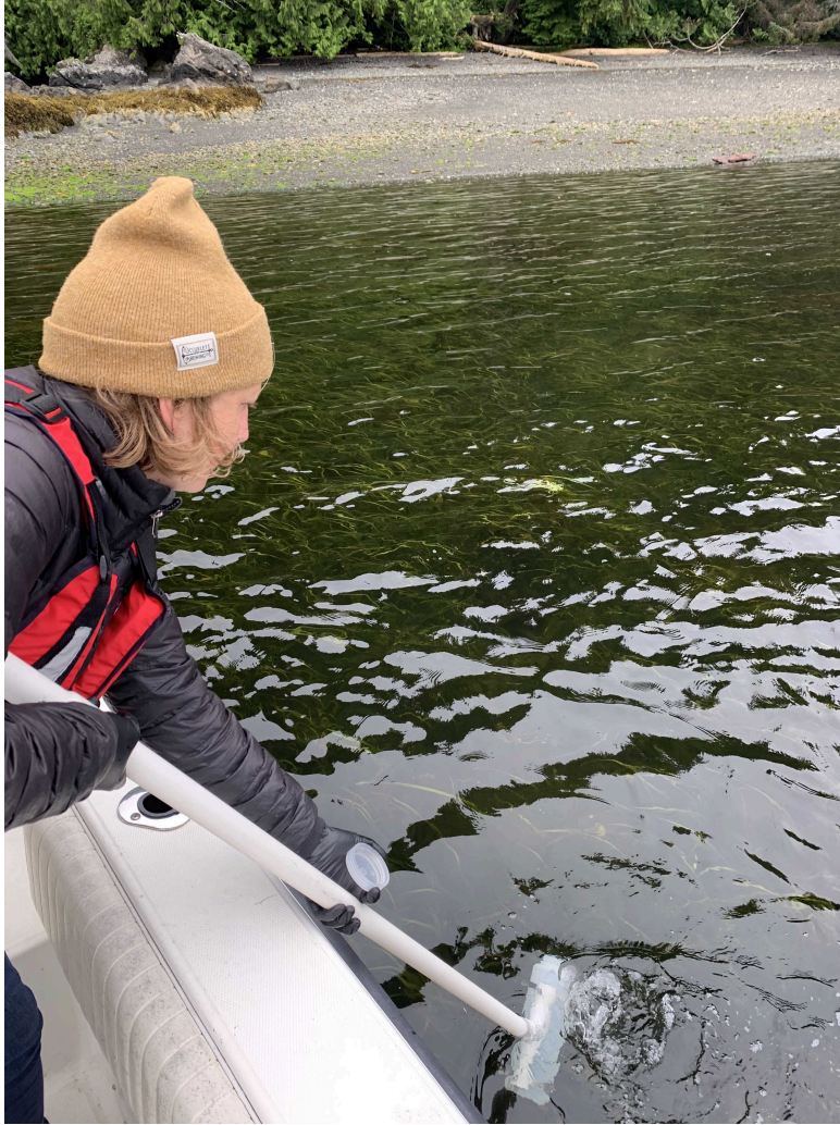
Fig. 3. Sampling seawater from a boat. Bottle has just been rotated to release bubbles.
