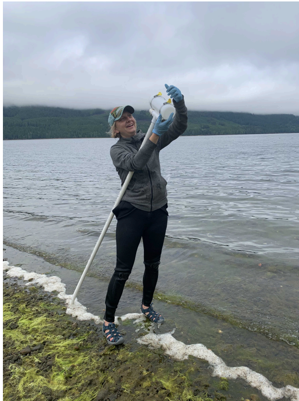
Fig. 2 Attaching the Nalgene for a wading-access sample.
