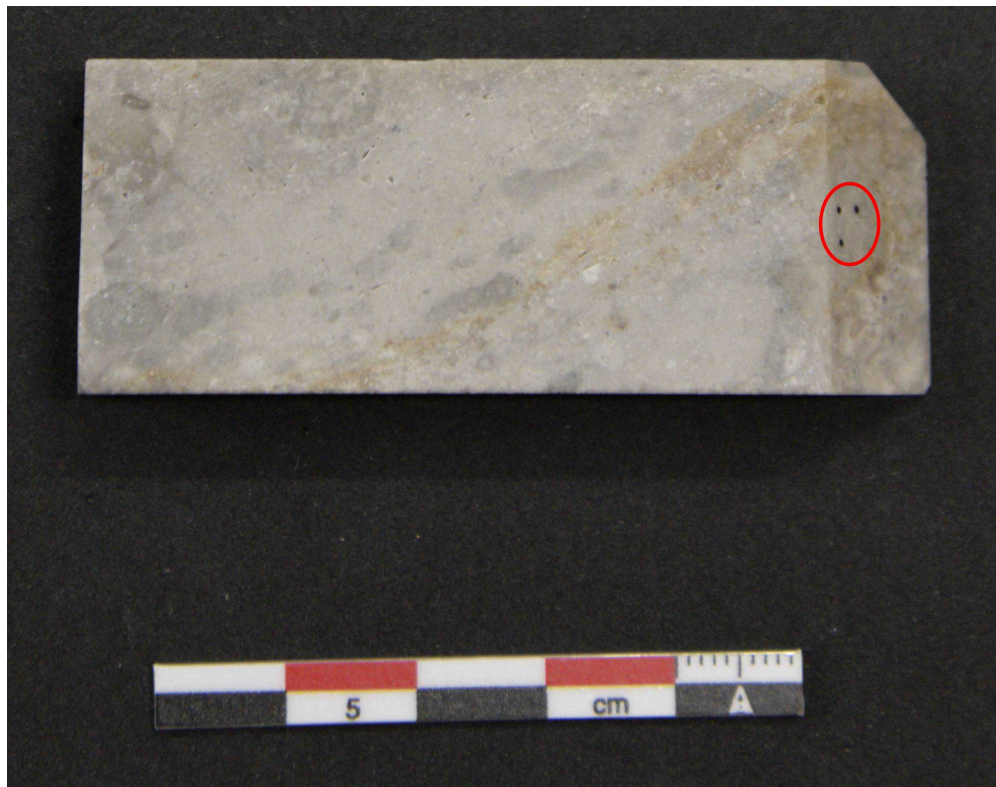
Final experimental standard sample with beads, view of side A (corresponding to the "dorsal" side of bifacial lithic artefact; here: flint).
