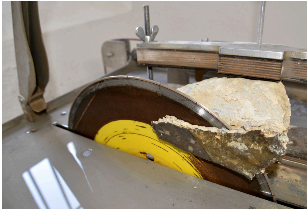
Cutting slice, with safety cover lifted for photo (here: flint).
