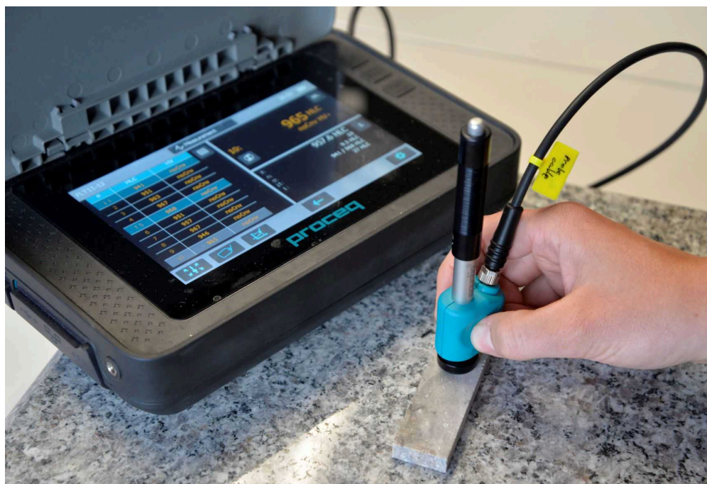
Measuring Leeb rebound hardness.
