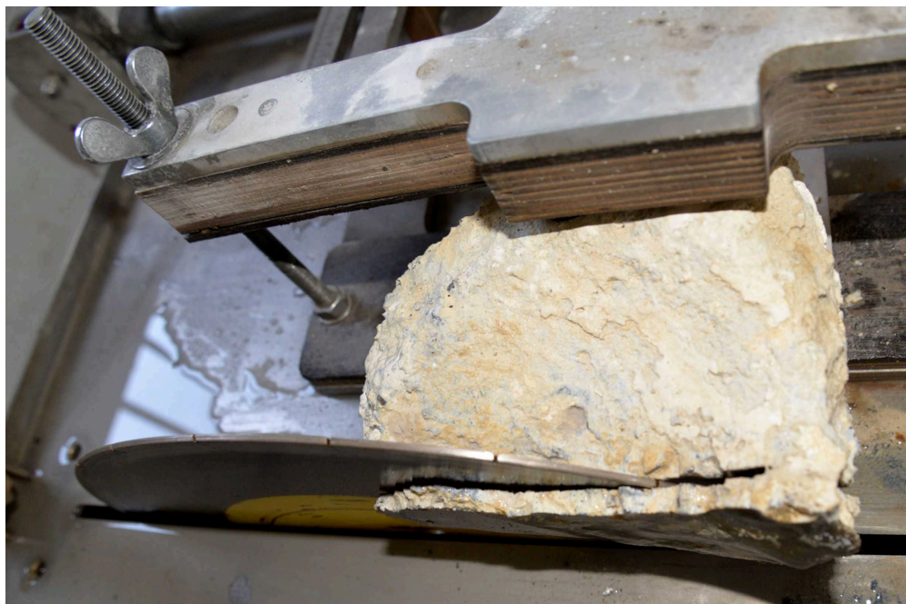
Cut to provide level surface, photo with safety cover lifted (here: flint).
