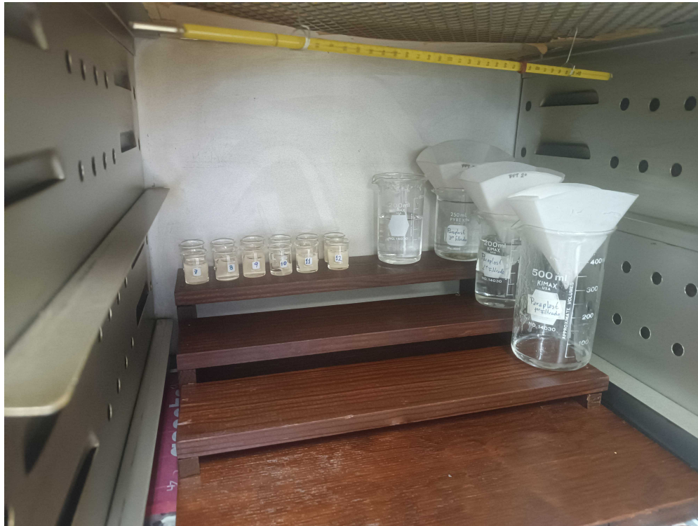
Figure 3. We remove the steel inner trays of the oven conformably handle the beakers. We use a customized wood base layered to get ready access to the beakers. A thermometer was hanged to monitor the temperature at a specific site of the oven.
