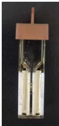
Figure 3. Sterile cuvette with a 0.1 cm electrode gap for electroporation (BIO-RAD).
