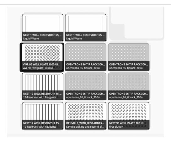
Placement of LABWARE and TIPS in the OT2 Deck used for the Omega Biotek Stool extraction protocol. These materials are for purifying 96 samples.
