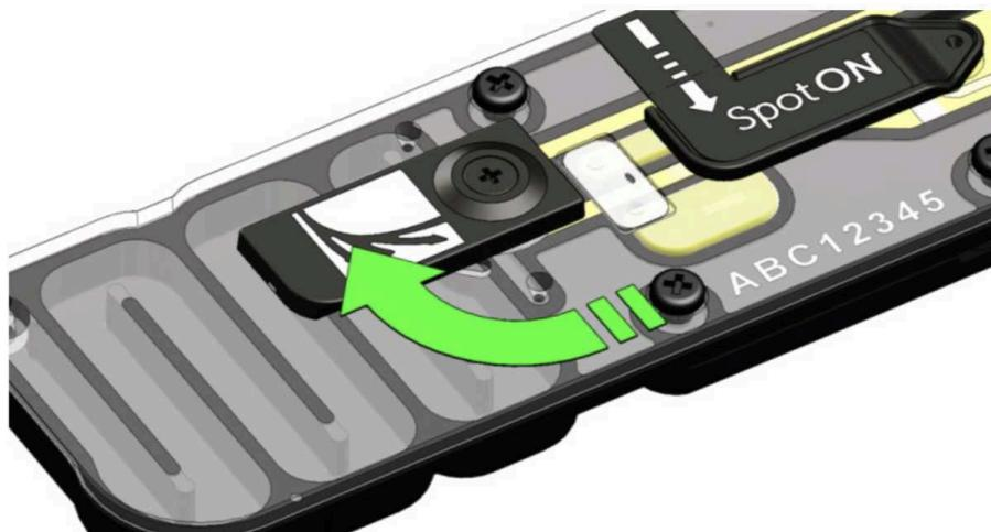
40 After opening the priming port, check for a small air bubble under the cover. Draw back a small volume to remove any bubbles:
