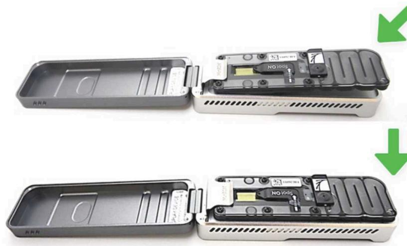
39 Slide the flow cell priming port cover clockwise to open the priming port.
