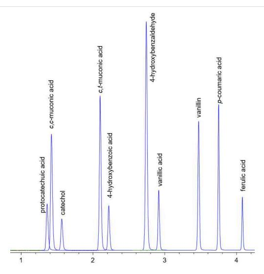
Elution order including muconic acid isomers and aromatic analytes analyzed using 'Aromatics Mix Large Rev. 1 Standard Mix'. Diode array detection wavelength signals are overlaid here to display analytes in elution order in one chromatogram
