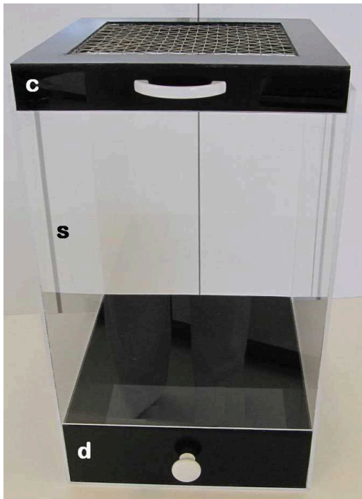
Figure 1. General view of the trial box for the inverted screen test. c: cover with the grille and climbing barriers; s: cover holding support; d: closed recovery drawer.
