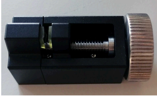
Fig. 1. The Vise Jig provided by Artec. Notice the soft plastic placed between the jaws, which will prevent the artifact from being damaged.
