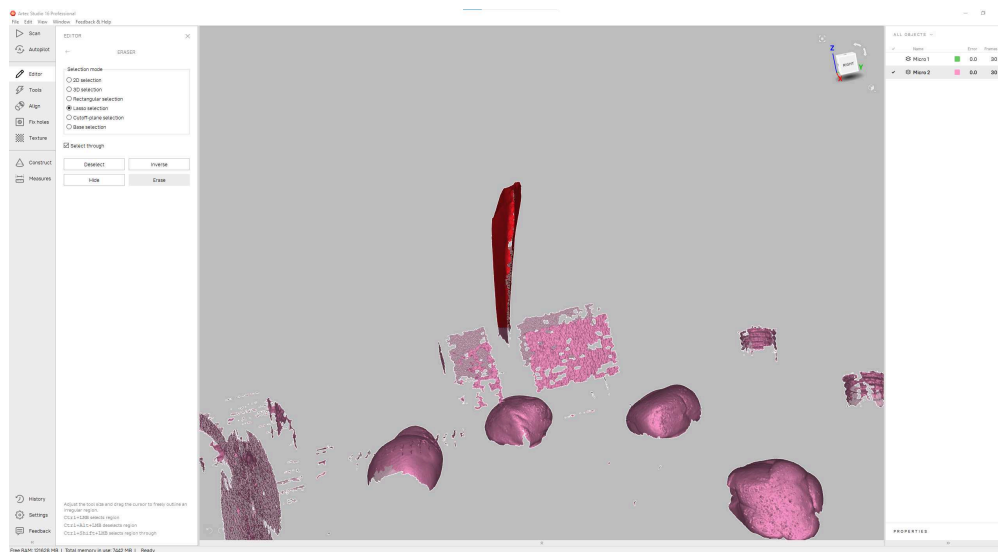
Fig. 9. Selection of the artifact with the Lasso function used to erase all unwanted parts of the scan after pressing Inverse and Erase .
