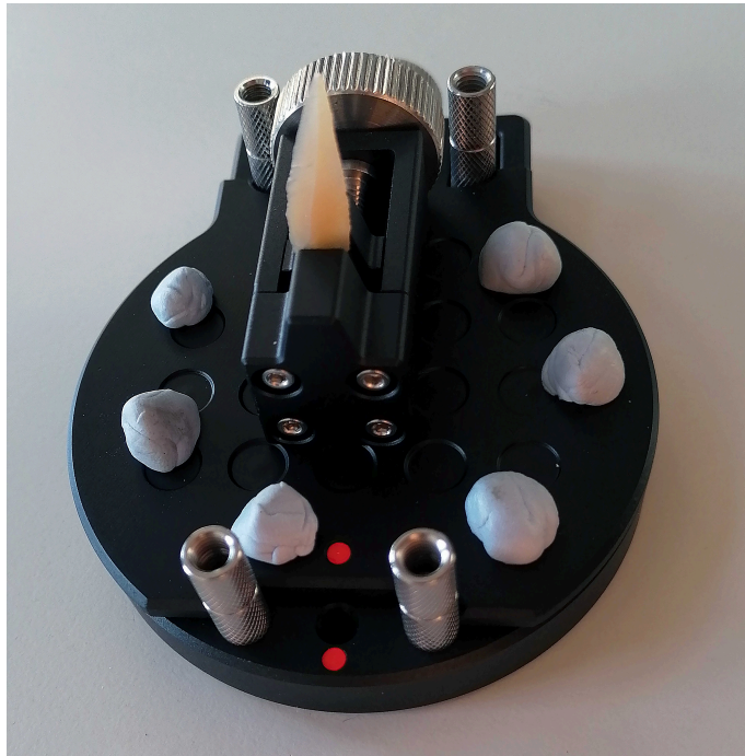
Fig. 2. The lithic artifact placed between the jaws of the Vise Jig and the adhesive putty attached to the Gum Jig used to create additional tracking features. In this case, the artifact is oriented according to the longitudinal axis with the proximal part at the bottom.
