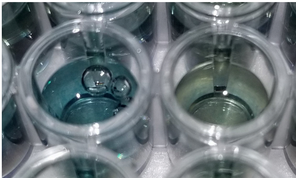
Fig. 11. Left: Well with air bubbles. Right: Well without air bubbles.
