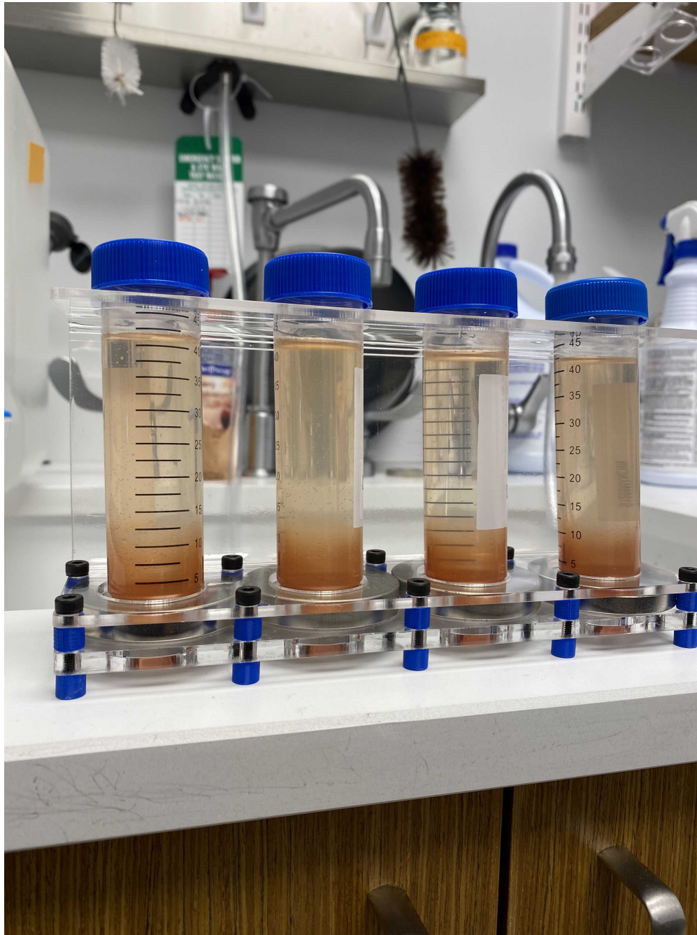
Conical tubes with wastewater samples after incubation on magnets. Notice the rust-red Magnetic Nanotraps that have precipitated at the bottom of the tubes near the magnets.
