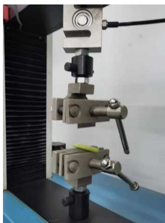
The shear tests of garlic scapes.
