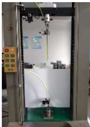
The garlic scape fractures under tensile loading.
