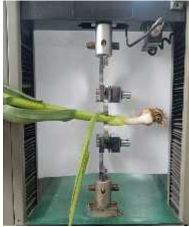
The compression tests of garlic plants.
