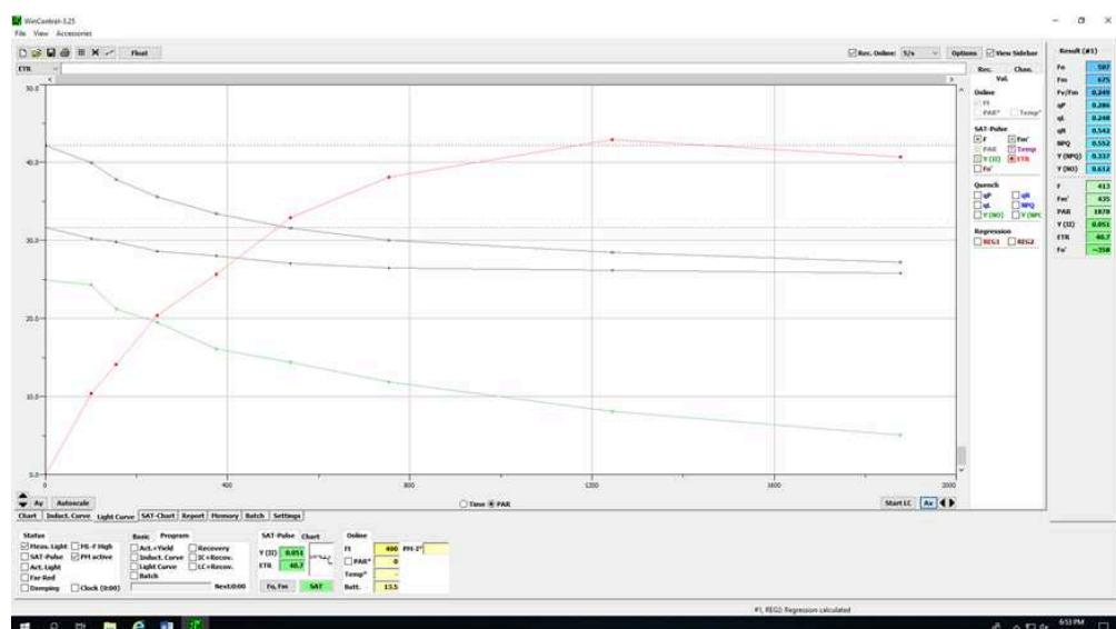
To achieve a successful RLC, there should be at least 3 points on the rise, multiple points to estimate the ETRmax, and at least one point on the decline at the highest irradiance (see instrument manual).
