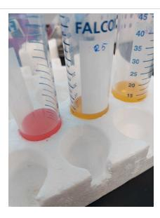
We have found that the optimal pH for the reaction between silicate and molybdate to form silicomolybdic acid is 3 to 4. Too low or too high pH decreases recovery of biogenic silica.
