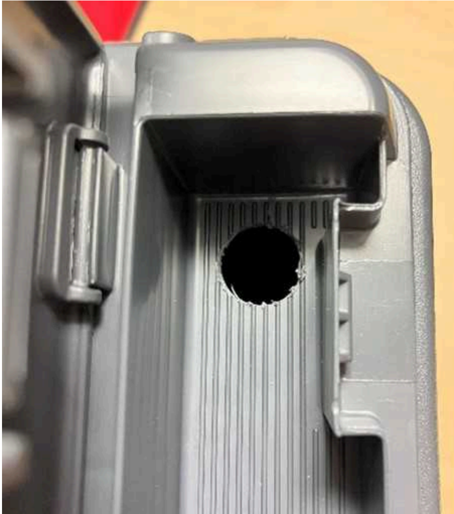
Figure 14. Recommended 13/16 inch drill location for rocker switch.
