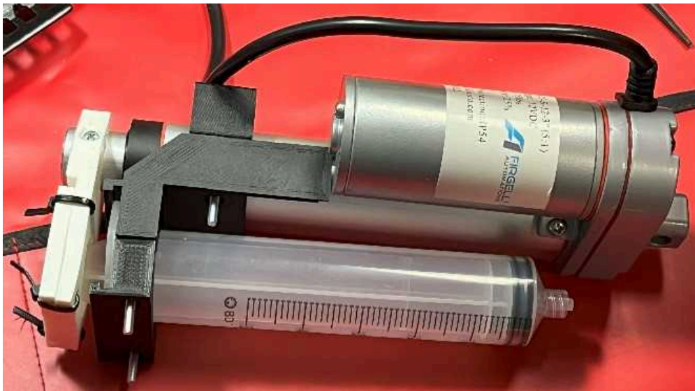
Figure 13. Syringe mounted onto the actuator using 3-D part #1. Ensure there is a gap between 3-D printed parts #1 and #4 on the flat or square side of the actuator.
