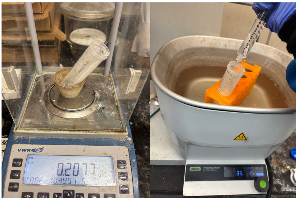
Lipase reaction set up. Left image: weighing lipase reagent into 50-mL Falcon tube. Right image: placing reagents into the Falcon tube and into the water bath.
