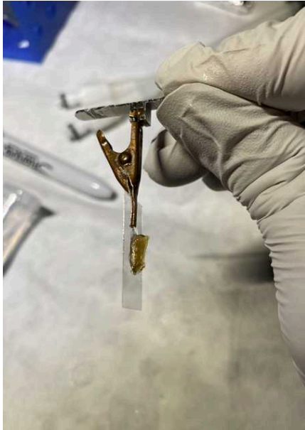
Fig. 7: Mounting Apparatus with Sample on Coverslip. The T-shaped mounting stub was glued to a copper electrical clip with fast drying epoxy. The clip may be used to pick up the glass coverslip with sample as shown. The sample was glued to the center of the coverslip as shown.
