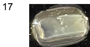
Fig. 2: After clearing and RI-matching, the sample should appear transparent.
