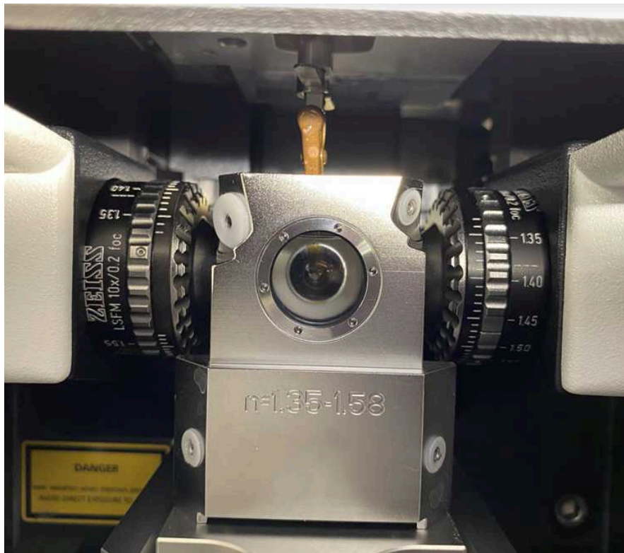
Fig. 12: How the sample should be mounted prior to imaging (20x). The sample should be directly facing the detection objective and perpendicular to the dual illumination objectives. The glass cover slip should be facing towards the front port window. 5x mounting will look similar, but with its respective chamber and lenses.
