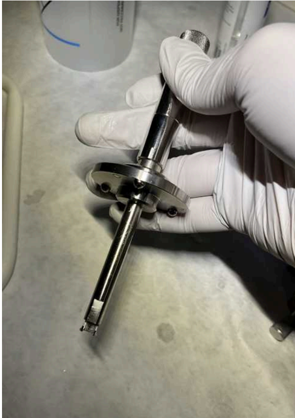
Fig. 8: The hook used to mount samples in the Light sheet 7. The hook may be inserted through the top of the Light sheet to grab the T-shaped mounting stub from above.
