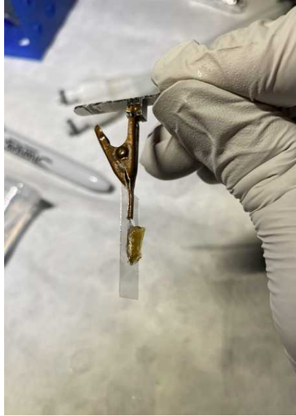
Fig. 11: Mounting Apparatus with Sample on Coverslip. The T-shaped mounting stub was glued to a copper electrical clip with fast drying epoxy. The clip may be used to pick up the glass coverslip with sample as shown. The sample was glued to the center of the coverslip as shown.
