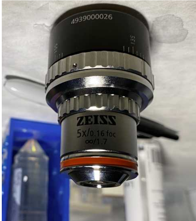
Fig. 6: Zeiss 5x/0.16 foc lens used as 5x detection objective.
