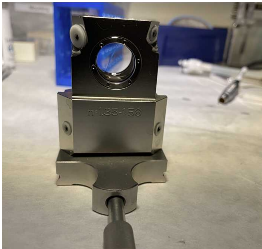
Fig. 15: n=1.35-1.58 R.I. 20x Imaging Chamber. Note that the rear port window is open to allow for imaging with an immersion lens.
