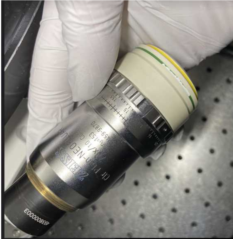
Fig. 13: Zeiss Clr Plan-Neofluar 20x/1.0 Corr n = 1.53 detection objective.
