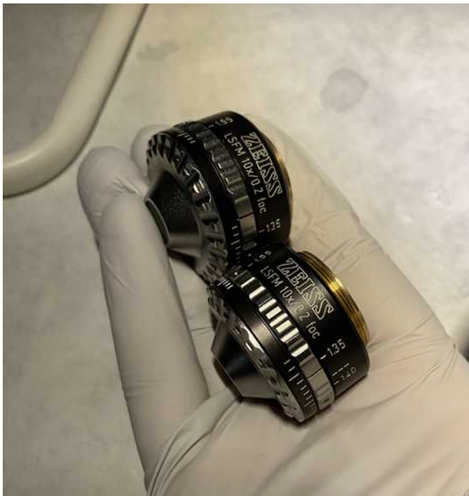
Fig. 14: Zeiss LSFM 10x/0.2 foc illumination objectives.
