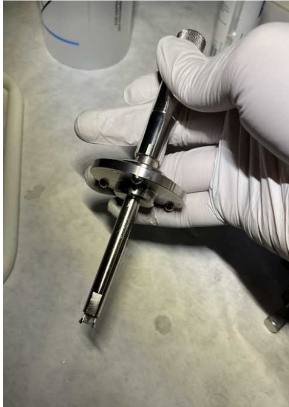
Fig. 12: The hook used to mount samples in the Light sheet 7. The hook may be inserted through the top of the Light sheet to grab the T-shaped mounting stub from above.
