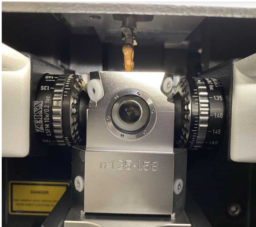
Fig. 16: How the sample should be mounted prior to imaging (20x). The sample should be directly facing the detection objective and perpendicular to the dual illumination objectives. The glass cover slip should be facing towards the front port window. 5x mounting will look similar, but with its respective chamber and lenses.
