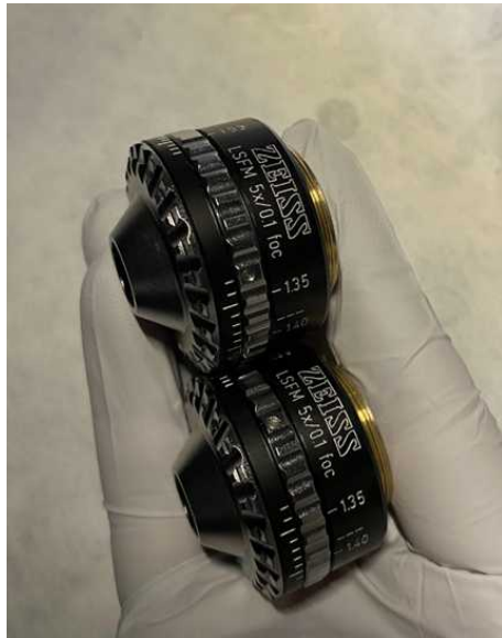
Fig. 7: Zeiss LSFM 5x/0.1 foc lenses used as illumination objectives.
