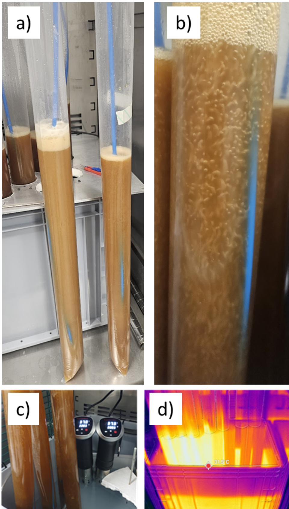
Bag set-up a) Bags removed from water bath for illustrative purposes, b) a typical bubble swarm and foam layer, c) close-up of the Bags in the water bath with heaters, d) a heat map showing water bath heating of the Bags.
