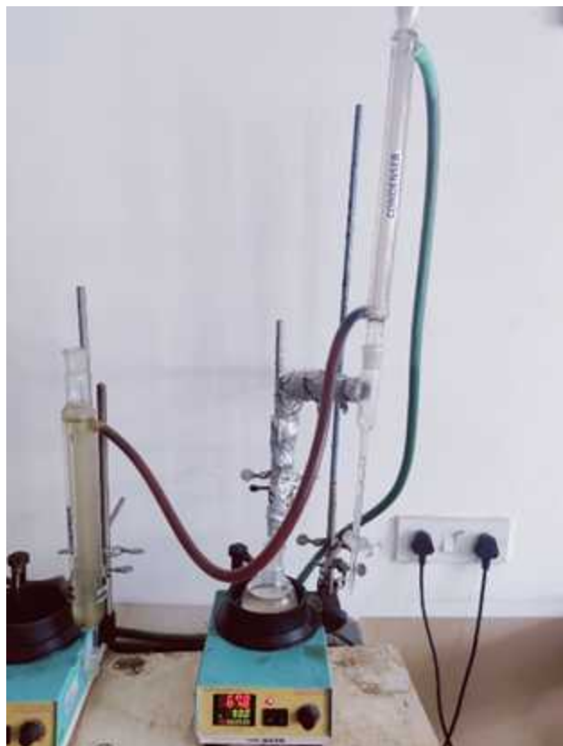
Refluxing using Dean-Stark apparatus and reflux condenser
