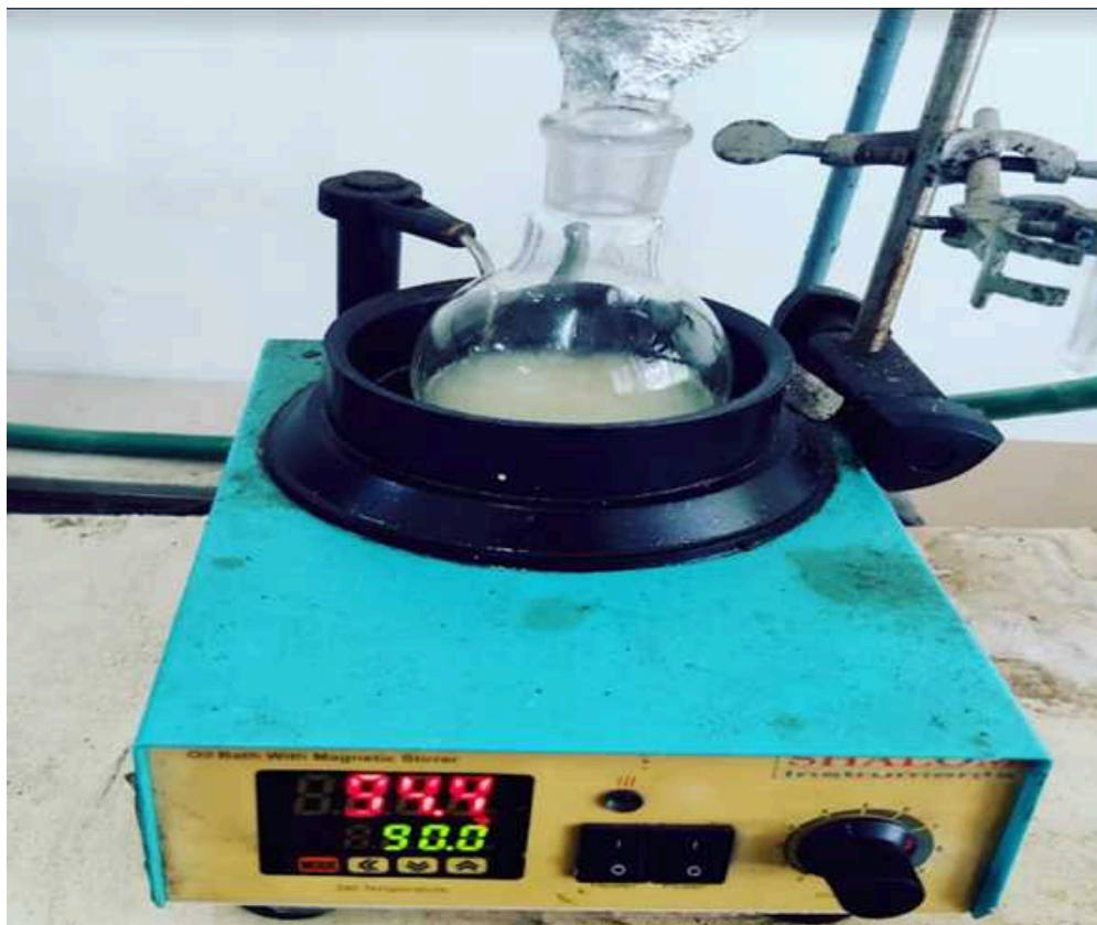
Refluxing using reflux condenser
