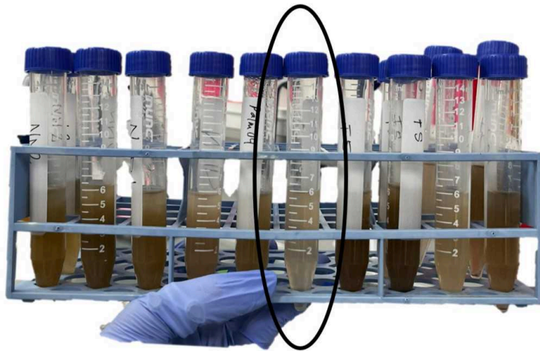
Figure 13. Colour chart for cell density dilutions, the sample in the black circle shows the colour for the correct dilution.
