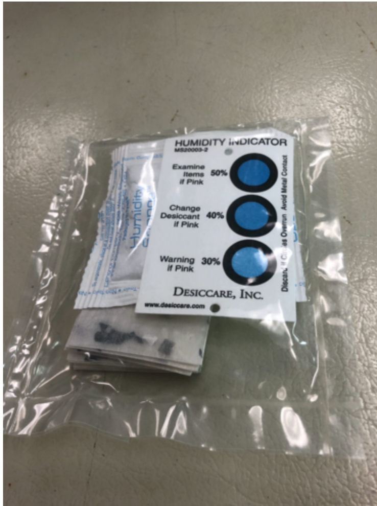
Figure 5. Dried cultures sealed with silica gel and indicator papers
