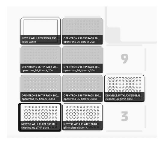
Placement of LABWARE and TIPS in the OT2 Deck used for the gDNA clean up protocol. These materials are for cleaning 96 samples.
