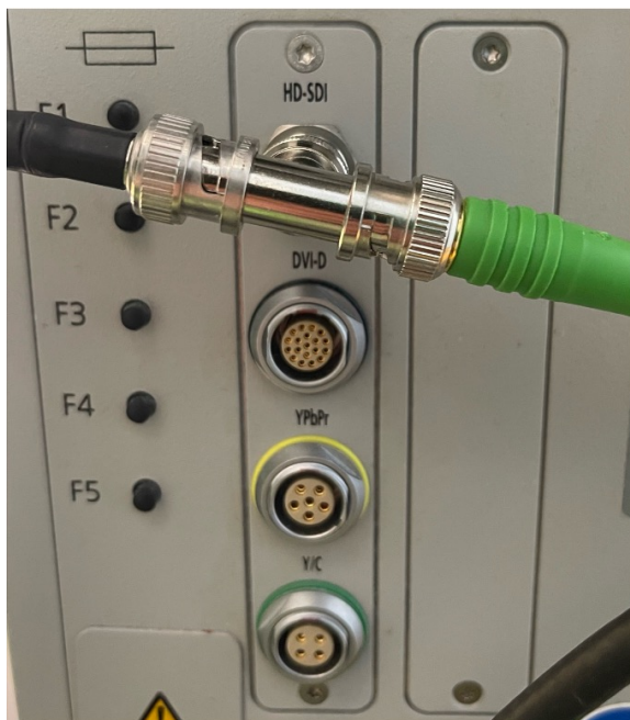
Microscope HD-SDI output after video splitter insertion with connecting cables attached.
