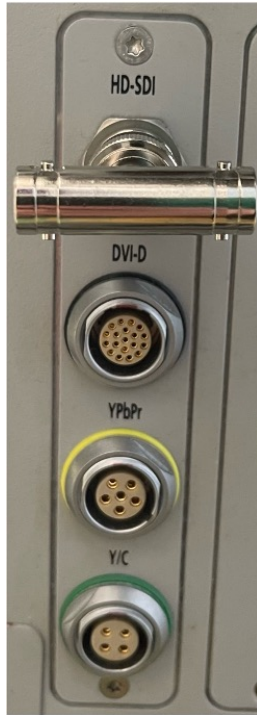
Microscope HD-SDI output after video splitter insertion.
