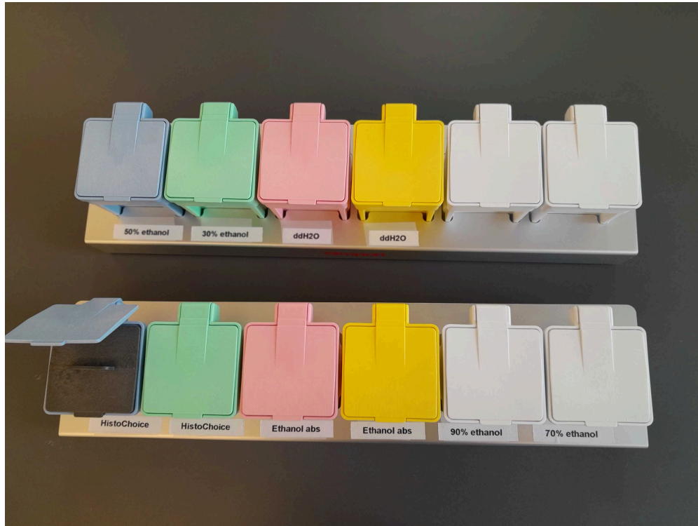
Fig. 1 | Slide staining station includes one anodized aluminum rack along with six assorted color jars (two white ones) and one slide staining rack. The aluminum holder can hold up to 6 staining jars. The anodized surface is resistant to rust, corrosion, and abrasion.
