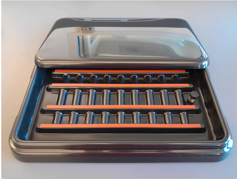
Fig. 5 | Humidity chamber with black lid for tissue incubation.
