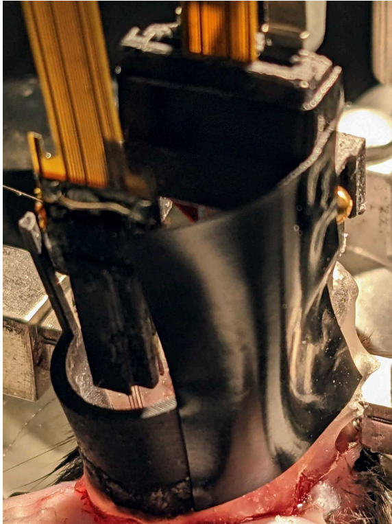
Ground/reference wires shielded by electrical tape.
