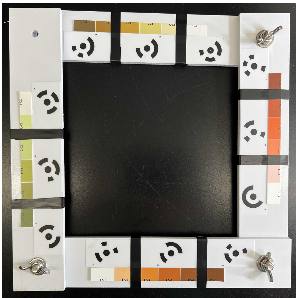
Completed V2 SCOU PR that incorporates 12 Metashape markers and all 4 CoralWatch Coral Health Chart color scales.
