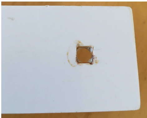
Back side of V1 SCOU PR hole. Square hole made by hand.
