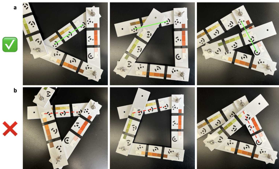
Figure 3. A) Proper SCOUPR set up to ensure intact scalebars (green). B) However, if one of the outtermost targets on the SCOPUR arms is covered, that particular scalebar will not be able to be used during model reconstruction and scaling (red, dashed line).
