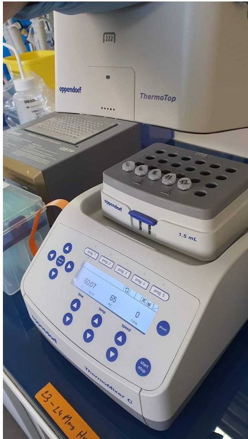
eppendorf Thermomixer with ThermoTop , 65°C 800RPM
