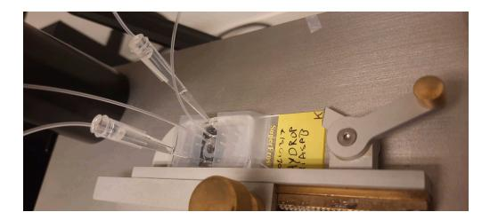
In this orientation, from north to south, you have the cell mixture, the oil, the outlet tube and finally the beads at the bottom.
