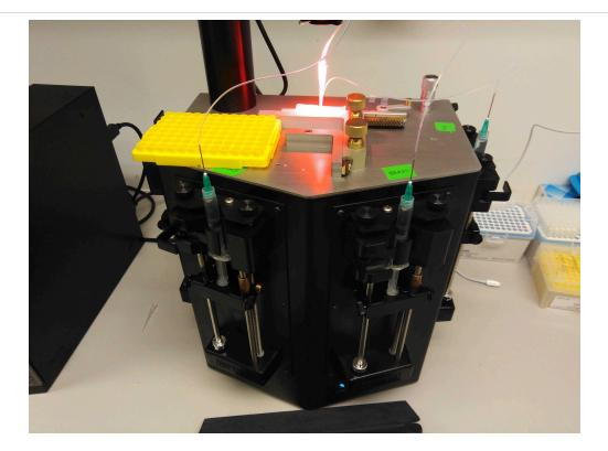
Note that we use a cover from a pipette tip box as a seating for the samples. For longer runs (10 minutes or more), we recommend that you use a small ice box or cold block to seat the samples as they are produced.
