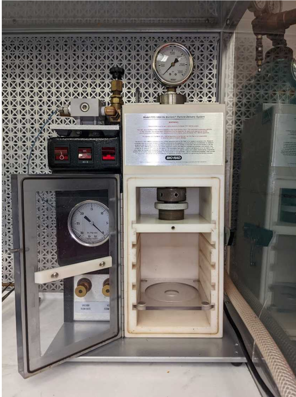
Figure 4. Assembly of the cartridge and rupture disc retaining cap, with plate shelf placed at the lowest position.
