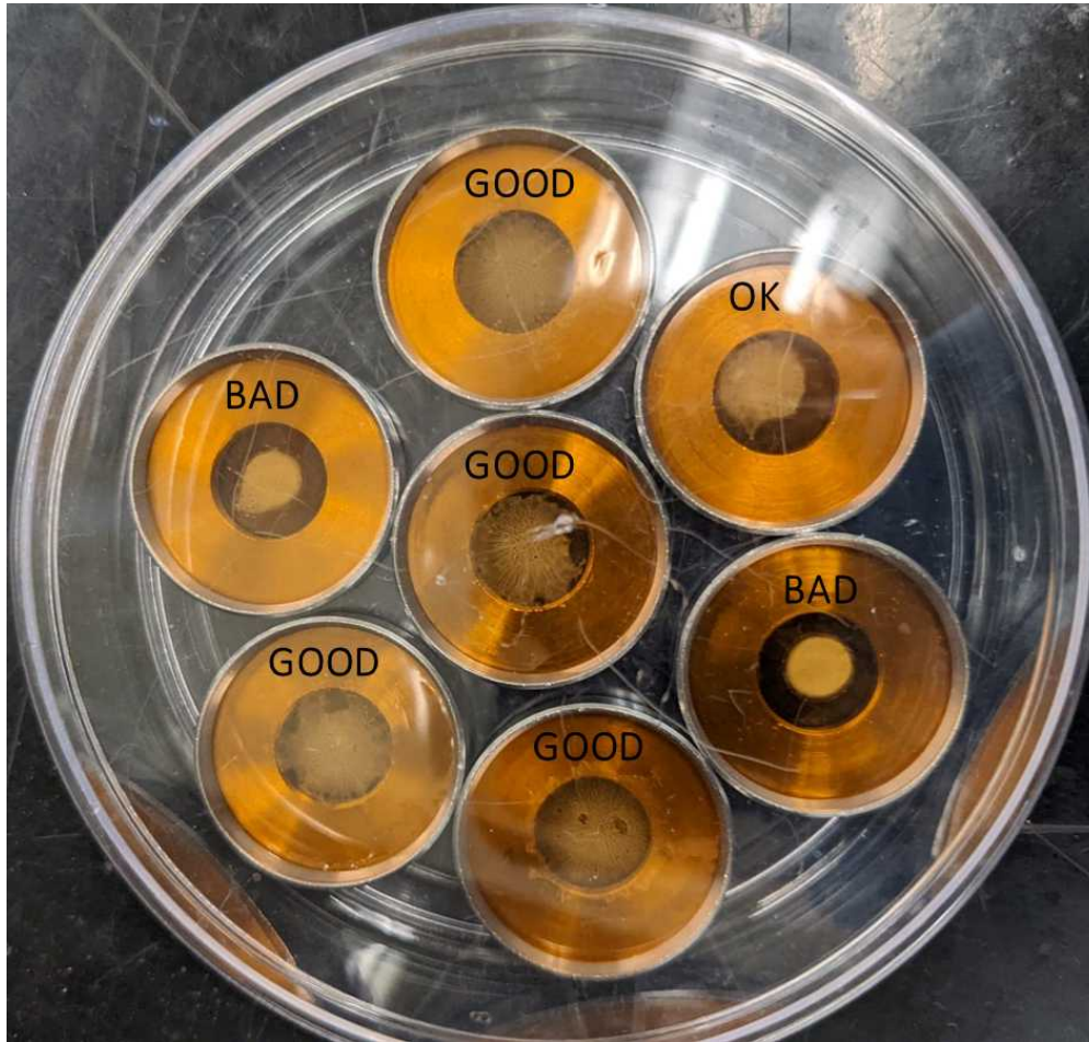
Figure 3. Macrocarriers with a range of gold spread. Gold spread evenly over the macrocarrier will have better transformation efficiency.
