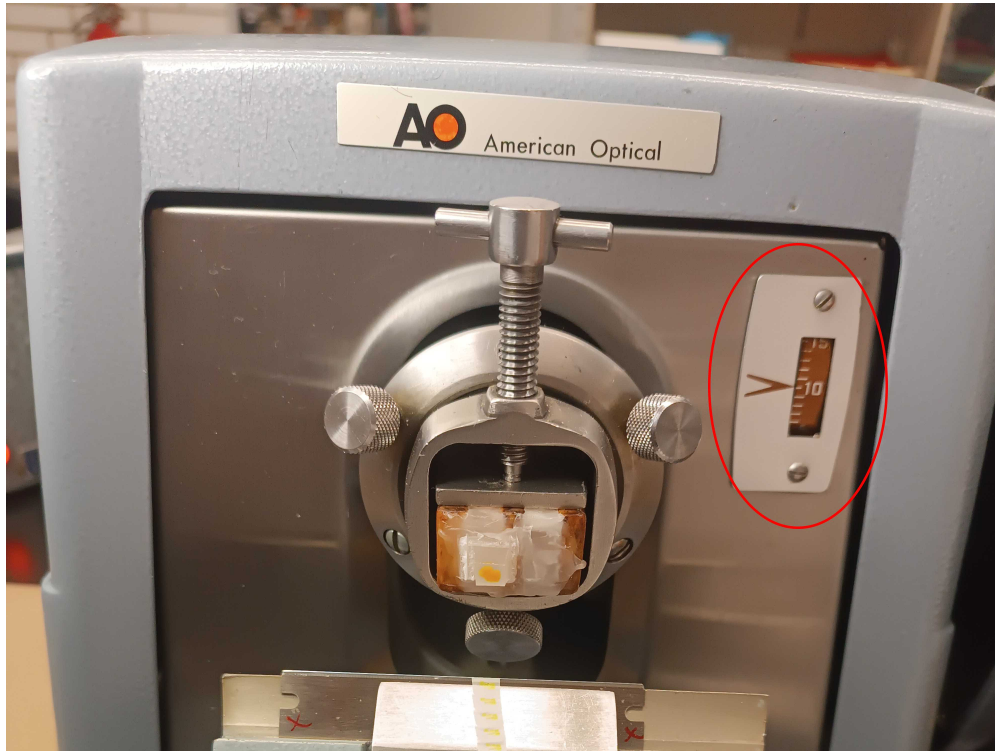
Figure 3. Before sectioning, the microtome is set to the desired section thickness (10 \mu\text{m} in this protocol) using the thickness control knob located at the rear of the instrument. The advance mechanism is fully reset by rotating the handwheel on the left side to its starting position, as the advance system has a fixed limit; reaching this limit during sectioning may interrupt the cutting sequence and result in tissue loss. Once adjustments are completed, the blade is positioned as close as possible to the surface of the paraplast block.
