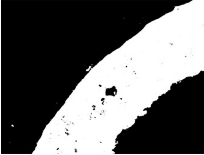
Background subtraction mask derived from saturation channel via saturation threshold value
