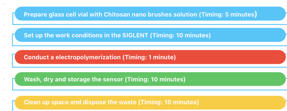
Figure 4. Process flow for the electropolymerization of chitosan nano brushes into the working electrode of a LIG sensor. The steps are separated into sections: preparation (blue), electropolymerization (red), stabilization and storage (green), and cleaning up the working area (yellow).
