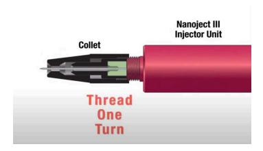
Nanoject III Injection Standard Collet/Chuck/Green Gasket.
