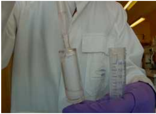
Figure 4 : Well insert the tip into the Sterivex to ensure the buffer does not overflow the cartridge.
