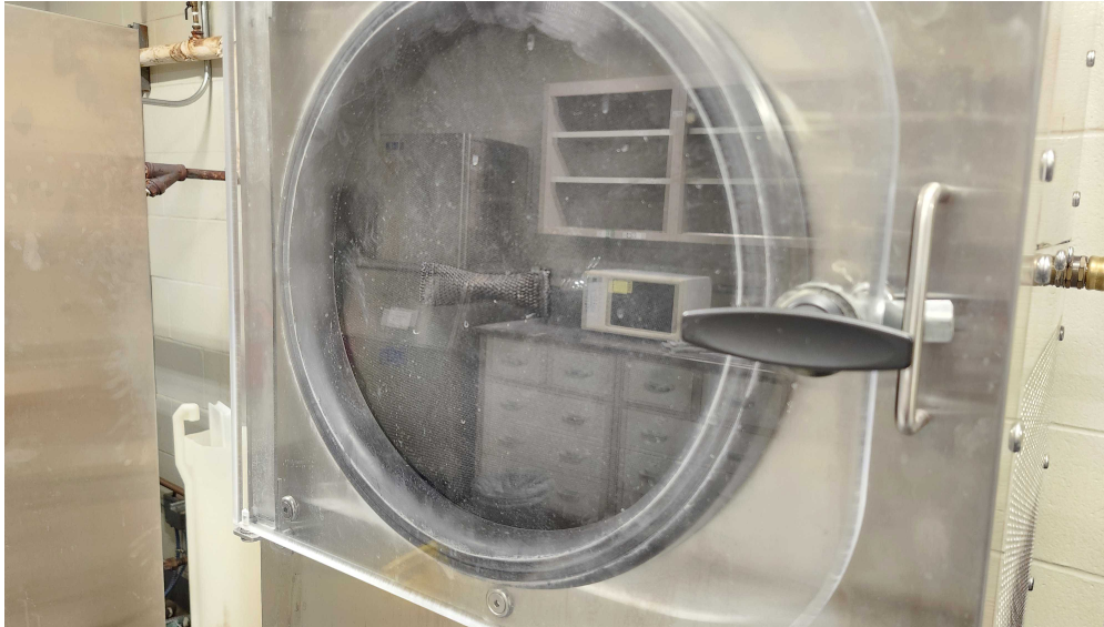
Closed freeze dryer with insulating cover and gasket installed
