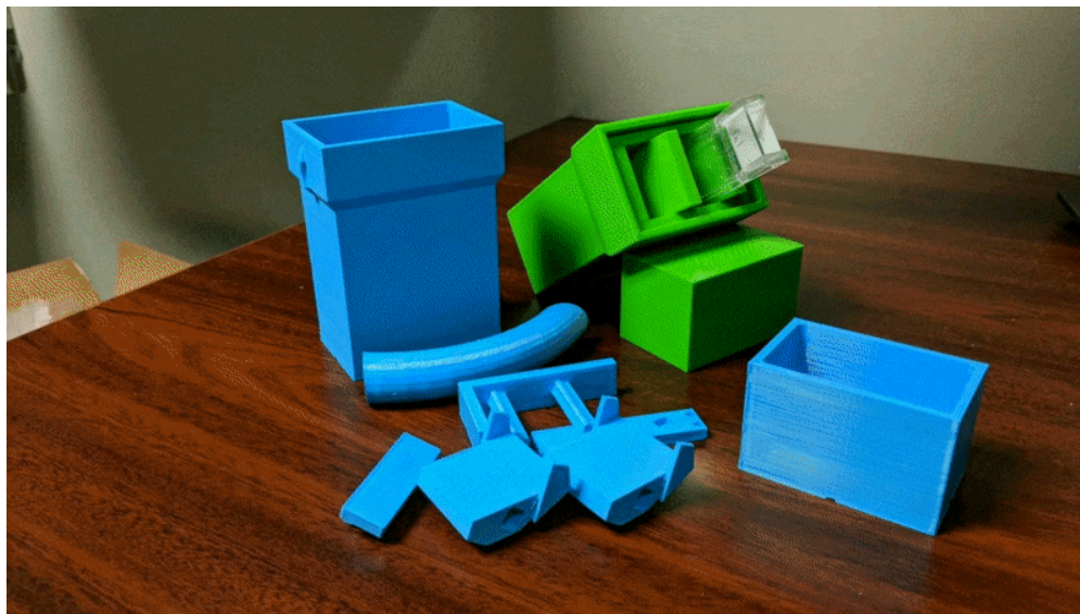
Assembly of the Inserts, + - Racks, and the End parts
