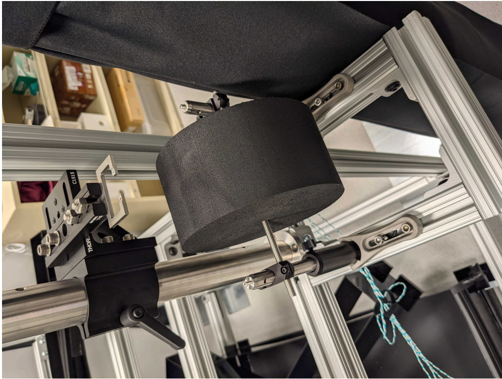
Completed headfixation apparatus, before positioning adjustments
