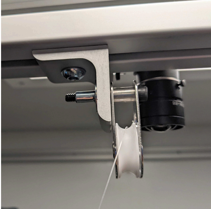
Center pulley mounted next to camera
