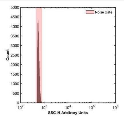
Example of threshold on the instrument noise floor
