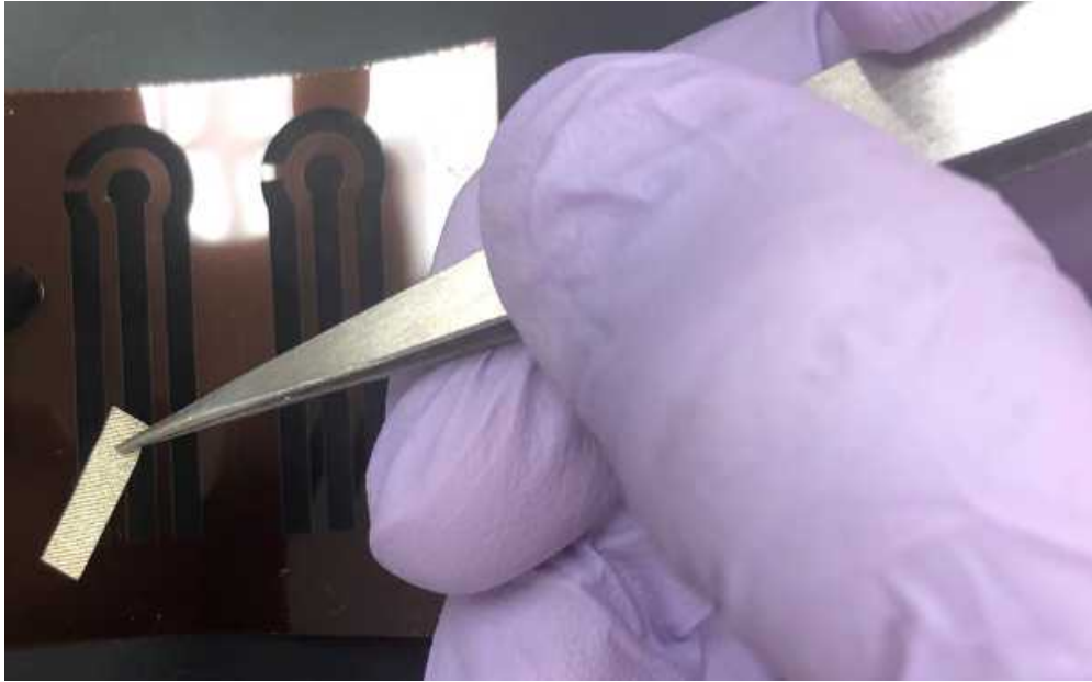
Figure 2. Photo demonstrating adhesion of polyester metal tape strips to bonding pad of LIG design. Each bonding pad corresponds to the working, counter, or reference electrode.
