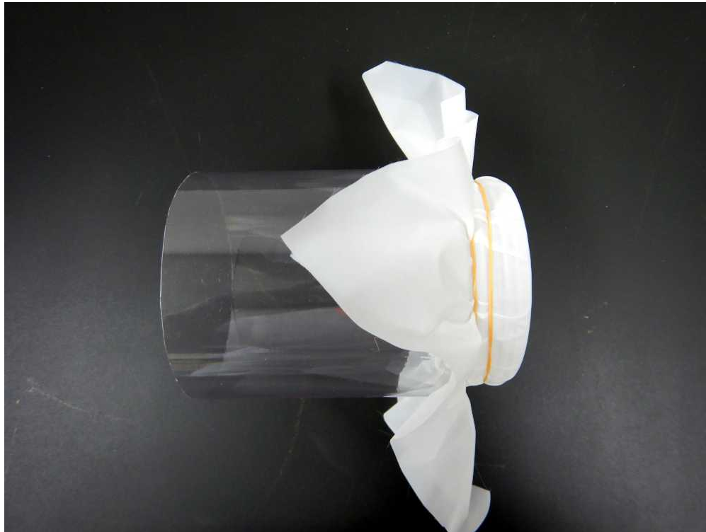
A completed filter.
