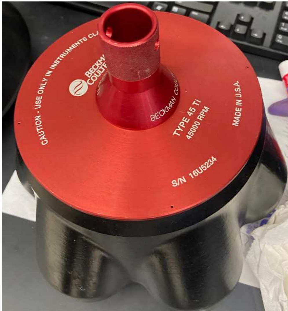
B.2. Ti-45 rotor for the ultracentrifuge tubes.
