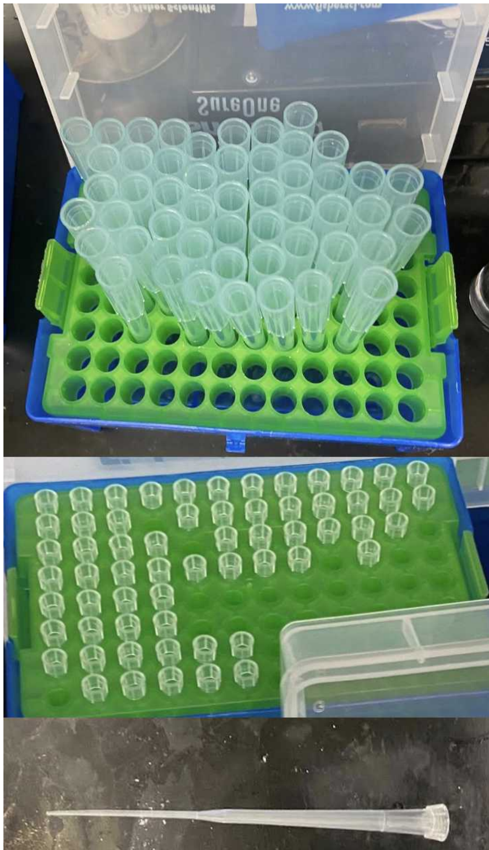
A.1. Micropipette tips. (Bottom image: gel loading tip)
