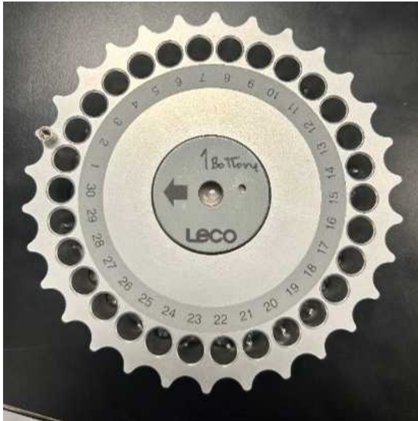
Figure 4. LECO carousel where samples are loaded.
