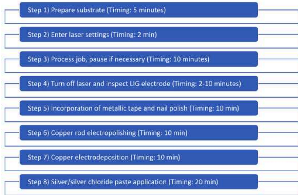
Figure 1: Process flow for LIG fabrication using NEJE mini laser.
